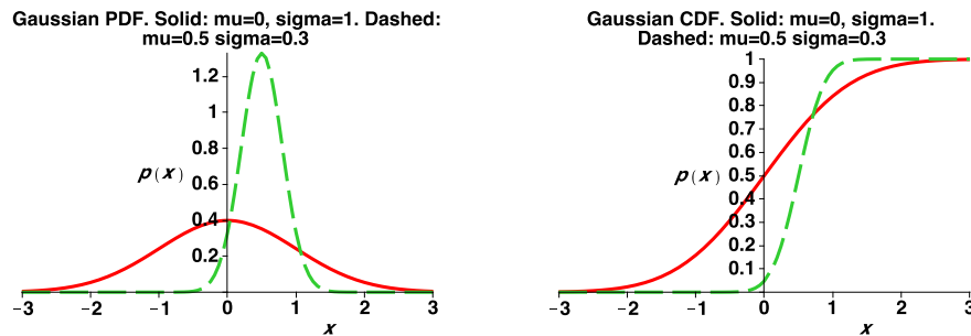
Fig. 16 Two examples of the Gaussian distribution, Eq. (219), for different choices of \mu, \sigma , and its corresponding cdf. The expectation value \mu controls the location of the pdf (i.e., when changing \mu the peak moves horizontally, without changing its shape), while the standard deviation \sigma controls its width (i.e., when changing \sigma the spread of the peak changes but not its location).
